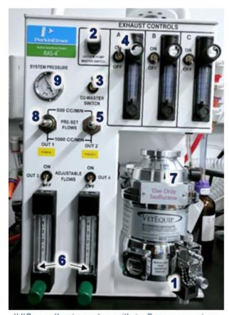
IVIS anesthesia system with isoflurane vaporizer
