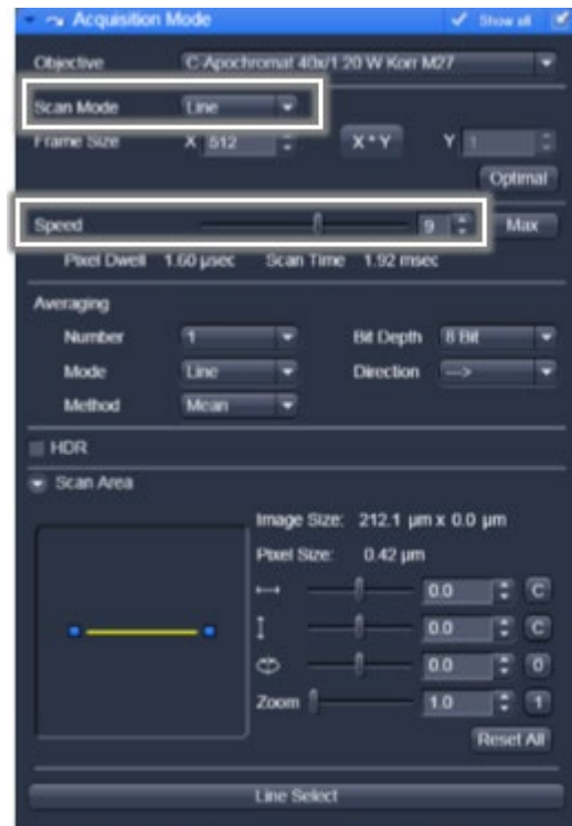
Fast line scanning acquisition parameters
