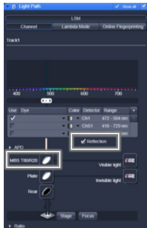
Light path configuration for Reflected light (Dichroic: MBS T80/R20)
