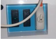
The front panel of the Vevo 2100 Imaging System features two passive and one active (rightmost) transducer ports. Transducer is in locked position.
