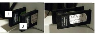
Diffusion (I) and neutral density, ND (J) filters pushed in (left) and pulled out (right)
