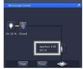
Condenser setup for DIC from Zen Locate tab
