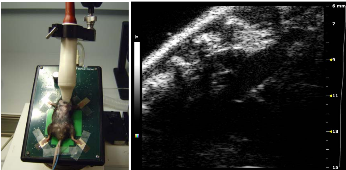
Figure 18. Image showing the positioning of the MS400 scanhead on a mouse to obtain a suprasternal view (L). B-Mode image of the suprasternal view (R).
