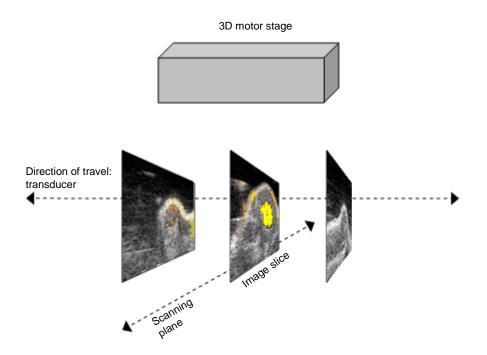
During the 3D data acquisition, the motor stage moves the transducer. Ensure that the animal under the transducer is flat in relation to the 3D scan direction to prevent unintended contact with the surface of the subject as the 3D motor stage moves the transducer.
