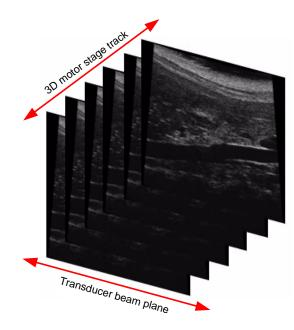
Each two-dimensional B-Mode, Power Doppler Mode, or Contrast Mode image slice is assembled with the other slices of acquired data and rendered by the Vevo software into a three-dimensional data set.
