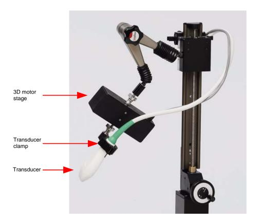
**3.** Lift the latch to open the clamp and then place the collar of the transducer in the clamp.
