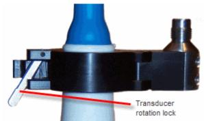
**5.** To set the transducer to any of the at the desired 90-degree angle in the clamp turn the transducer until you feel the collar snap into position.
