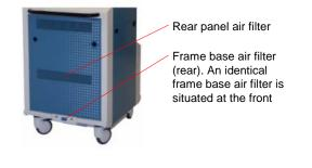
**WARNING**: Do not obstruct or block the filter inlets; overheating of the electronics could occur.
