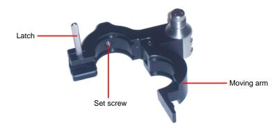
**4.** Close the moving arm of the clamp and then pull the latch down to the 45° notch. This transducer rotation lock setting holds the transducer but provides enough freedom for your to rotate it.
