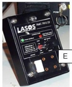
Argon laser flip switch: up to activate, down to put on standby
