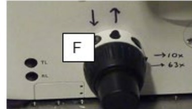
Focus knob on the right side of microscope. Arrows above buttons show quick one-push movement of objective
