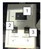
Startup switches 1-Main, 2-System/PC, and 3-Components
