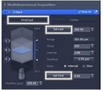
Tool to setup z stack by First/last focus positions
