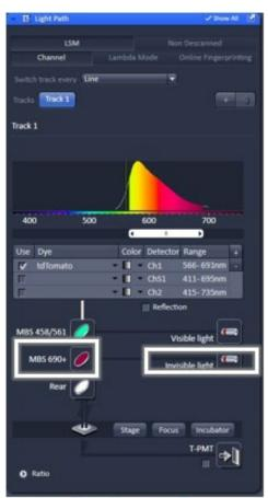
Light path configuration for multiphoton excitation includes setting up the right dichroic filter (MBS690+ or MBS760+)
