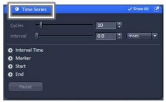
Time series tool to setup number of cycles and acquisition interval
