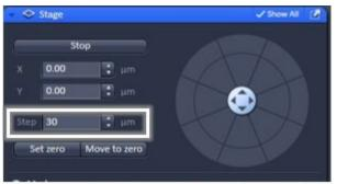
Stage tool for x, y adjustment of stage position
