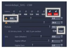
Multiphoton excitation wavelength can be tuned between 680 to 1300 nm. Pinhole aperture is set at Maximum.
