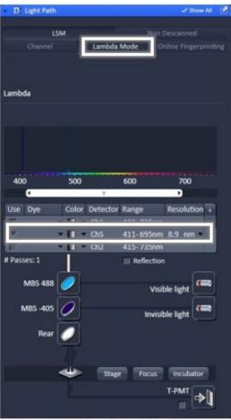
Sample Light path configuration for spectral acquisition by Lambda mode
