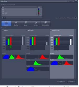
Smart Setup with suggested acquisition configurations for a given set of fluorophores
