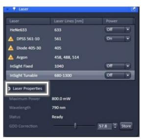
Laser tool for software control of lasers
