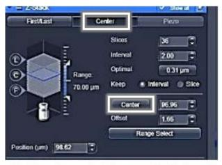
Tool to setup z stack by manual selection of center slice
