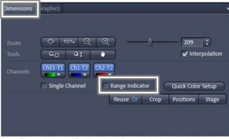
Range Indicator Tool to check image brightness saturation
