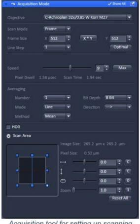
Acquisition tool for setting up scanning parameters
