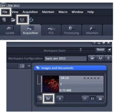
Saving images using main toolbar (Top) or via file handling area (Bottom)
