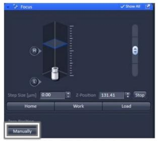
Tool to setup zero focus position
