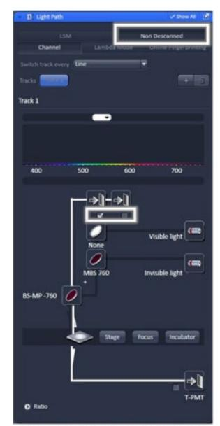
Light Path configuration for Non-descanned detection
