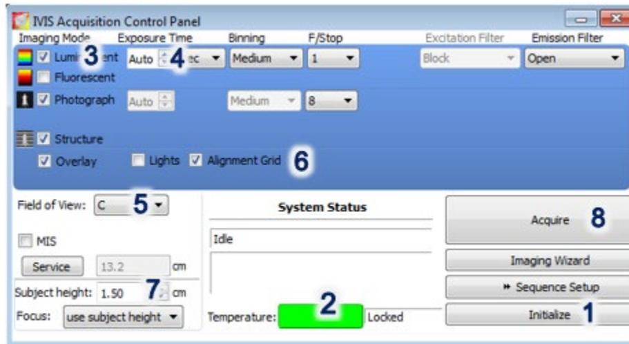
*IVIS Spectrum control panel provides the image acquisition functions.*
