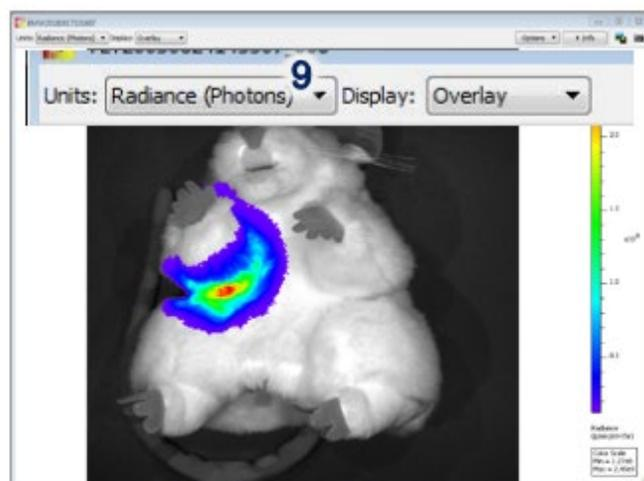
*Image window displays an overlay of photograph and luminescence with features relevant to an acquired image. The Units and Display option tools are zoomed in.*
