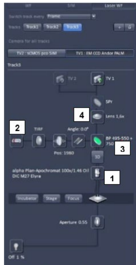
Light Path configuration for PALM/STORM/TIRF
