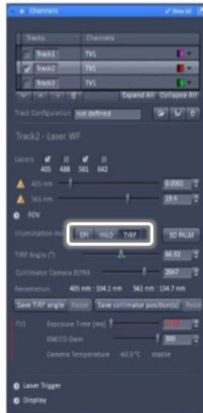
Channels tool shows multi-track setup, laser power, illumination mode (in box: Epi, HILO, TIRF) & other acquisition parameters
