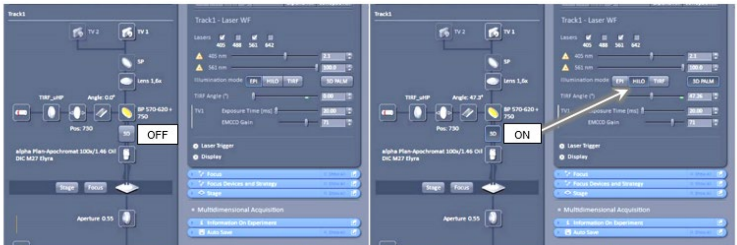
Light Path setup shows the 3D button to set PALM slider in position (when ON). The HILO button is selected when doing 3D PALM.
