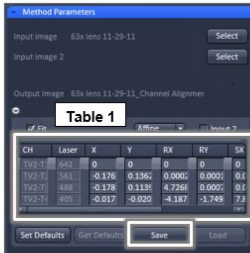
*Image processing: Calibration values obtained after application of Affine (or Lateral) fit*
