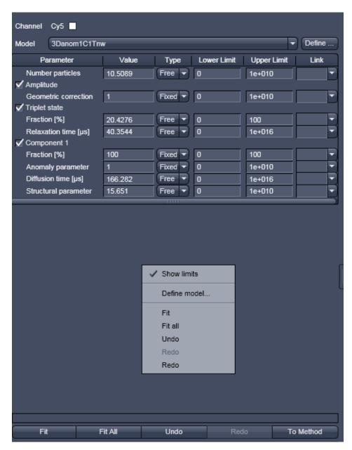
Fig. 452 Fit table with the Show limits menu activated in the context menu
