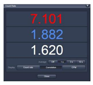
Fig. 411 Count rate window with correlation display
