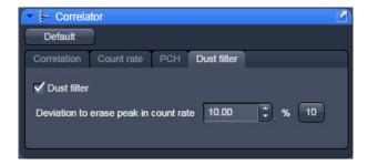
Fig. 364 Correlator tool - Dust filter active
