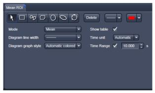
Fig. 758 Mean of ROI View Option control block
