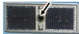
*Lock notch on transducer port*
