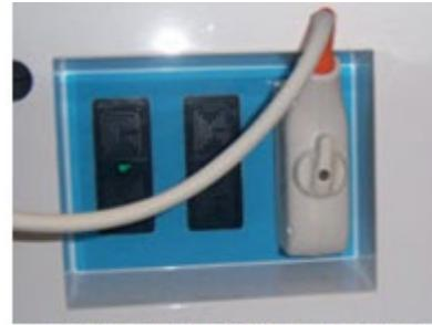
*The front panel of the Vevo 2100 Imaging System features two passive and one active (rightmost) transducer ports. Transducer is in locked position.*
