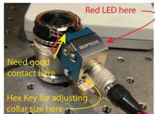
Setting up objective heater around objective
