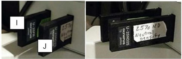
*Diffusion (I) and neutral density, ND (J) filters pushed in (left) and pulled out (right)*
