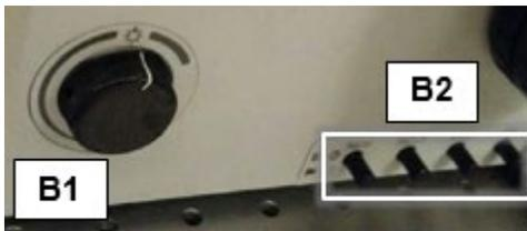
Brightness Adjustment knob (B1) and ND filters (B2)
