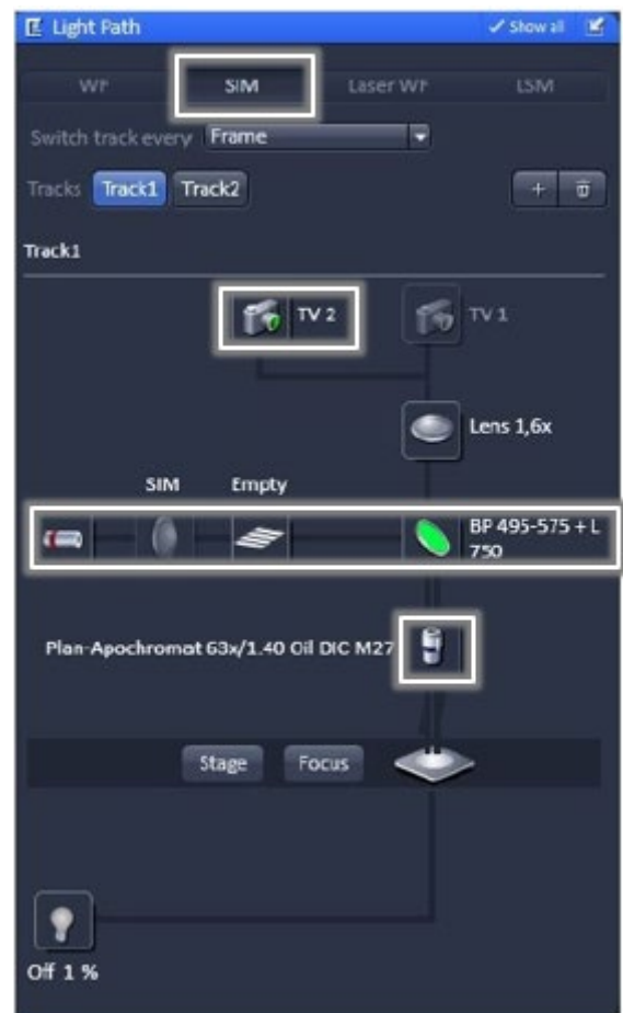
Light Path for configuring a SIM experiment
