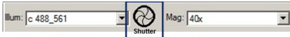
Illumination and Magnification settings. Opening the shutter is necessary to view sample thru eyepieces.
