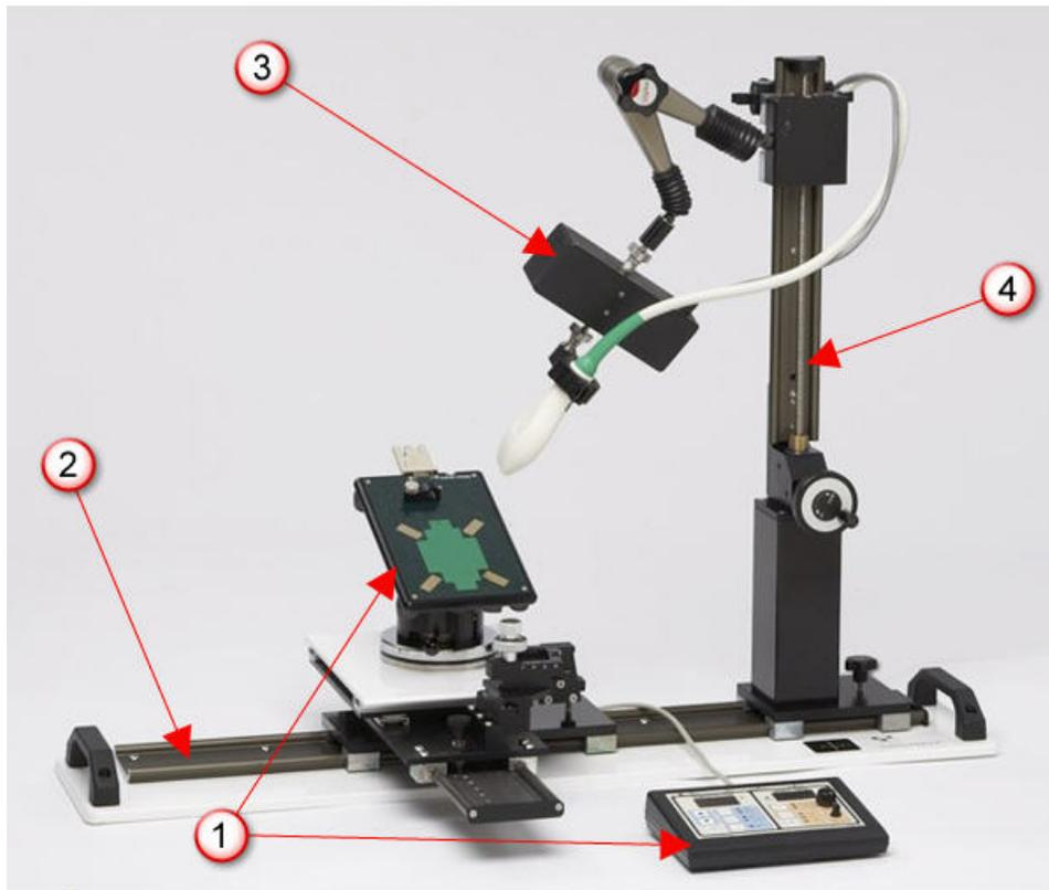
*Vevo Imaging Station Operator Manual including the injection system and 3D motor system*
