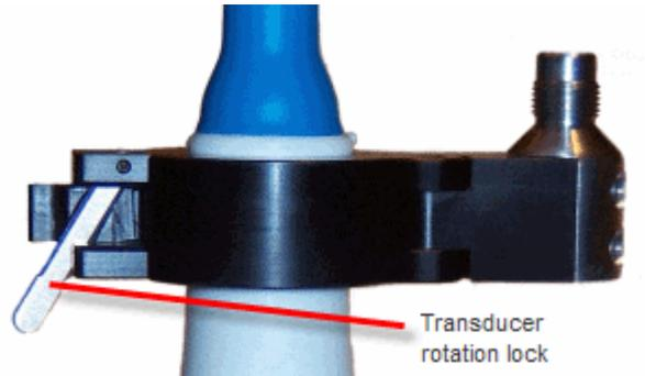
5. To set the transducer to any of the at the desired 90-degree angle in the clamp turn the transducer until you feel the collar snap into position.
