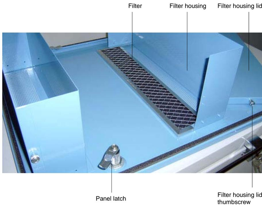
5. Slide the filter from the filter housing.
