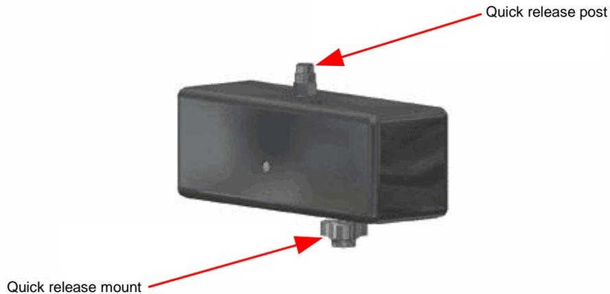
2. Carefully line up the holes on the post with the pins on the quick release mount.
