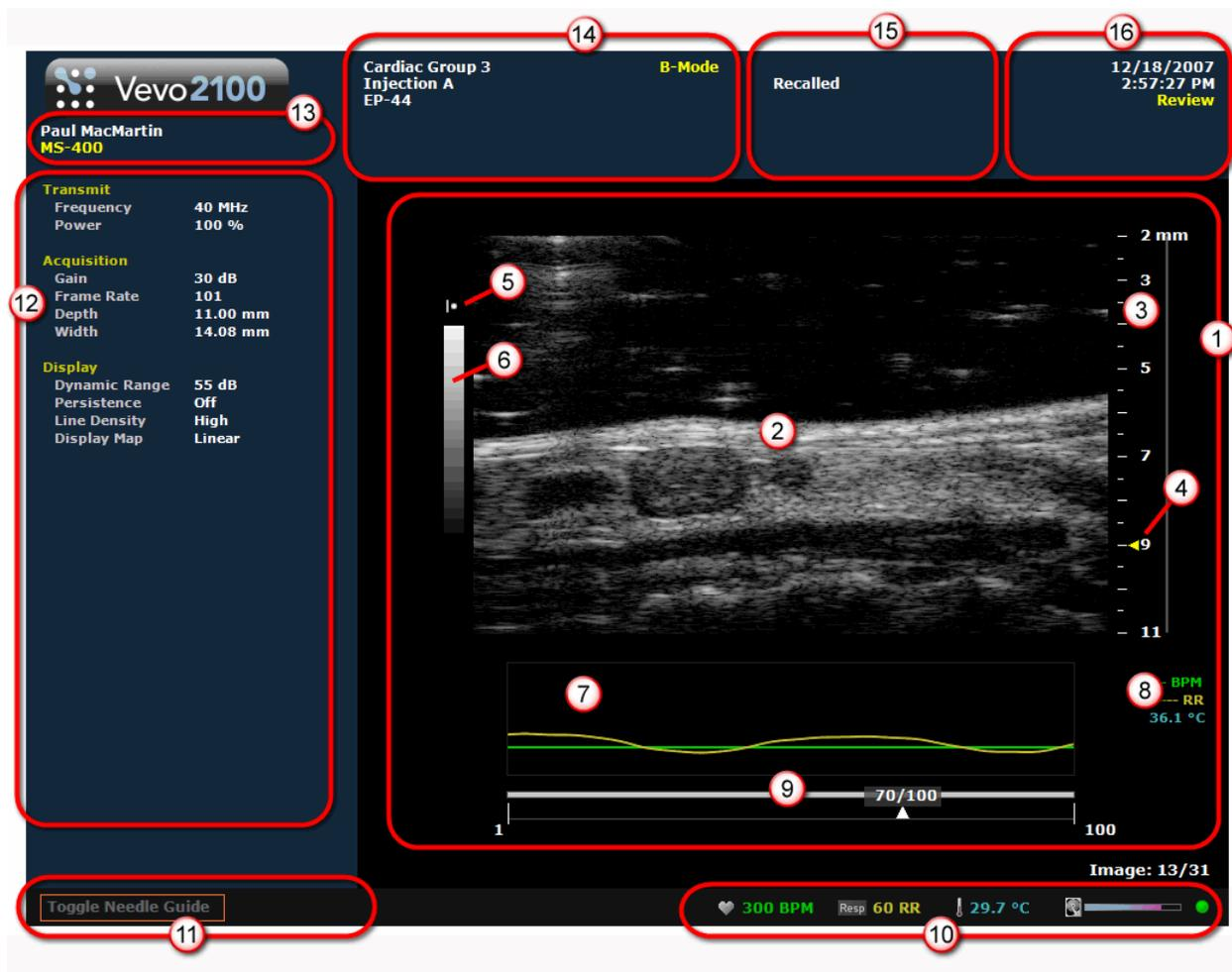
A typical Mode window workspace. This example is a B-Mode window displaying a stored cine loop.
