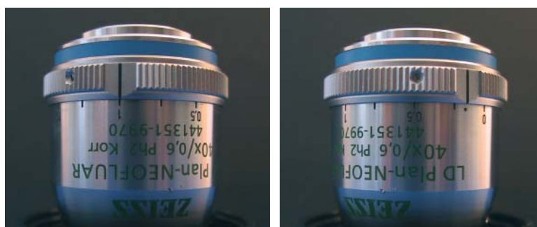
Regular glass slide (1 mm thick) => 1, thin slide (0.17 mm thick) => dot, DuplexDish and FrameSlide => between dot and 0.
