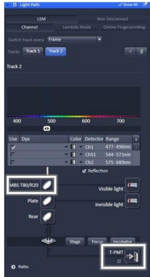
Sample Light path configuration for reflected light (Ch1) and transmitted light (T-PMT)
