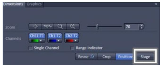
*Stage option for manually selecting different stage positions from a tiled image*
