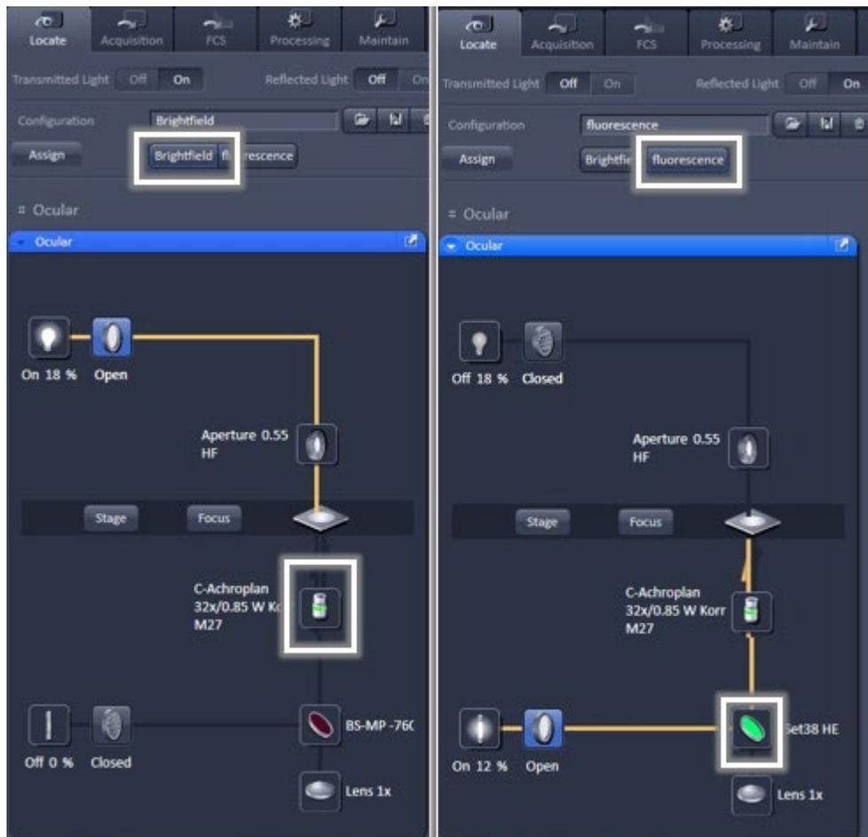
Light path to view sample thru eyepieces: L - Brightfield, R - Fluorescence
