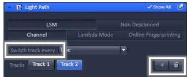
*Tool for scanning sequential acquisition configuration: by Line or by Frame*
