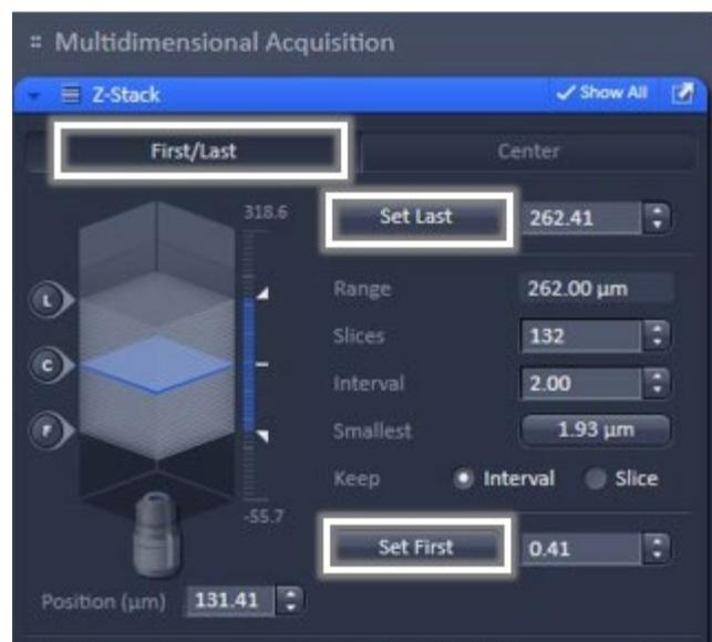
*Tool to setup z stack by First/last focus positions*
