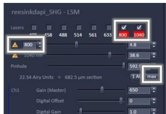
Multiphoton excitation wavelength can be tuned between 680 to 1300 nm. Pinhole aperture is set at Maximum.
