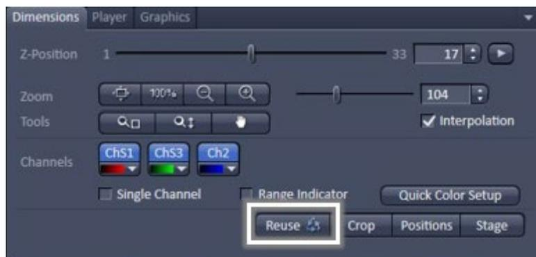
*Reuse tool opens up previously used acquisition and scanning configurations*
