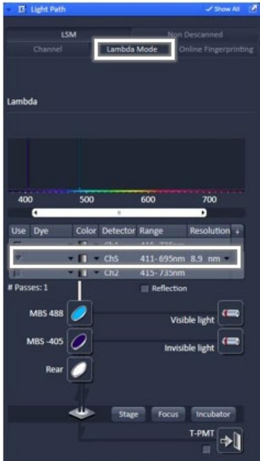
*Sample Light path configuration for spectral acquisition by Lambda mode*
