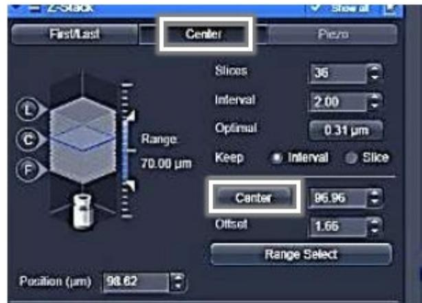
*Tool to setup z stack by manual selection of center slice*
