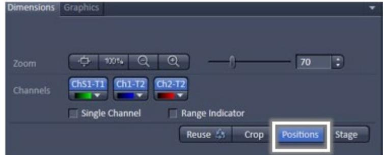
*Positions option for manually selecting different positions from a tiled image*
