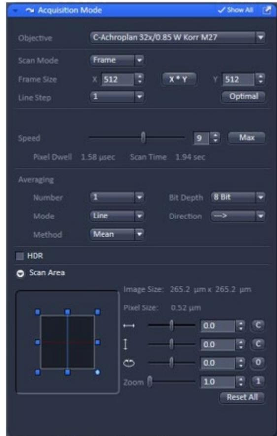
*Acquisition tool for setting up scanning parameters*
