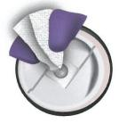
Pipette the reference into the sample port. See pipetting tips on reverse.
