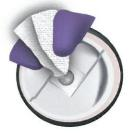
Pipette sample into the sample port. See pipetting tips on reverse.
