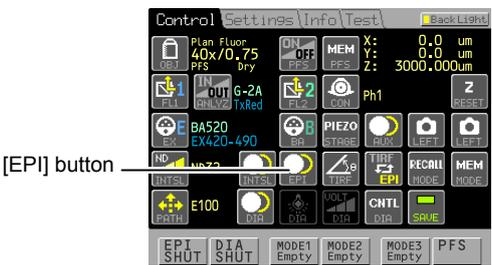
1. Pressing the [EPI] button (EPI shutter) on the [Control] screen, toggles the motorized shutter for episcopic illumination open and closed.
