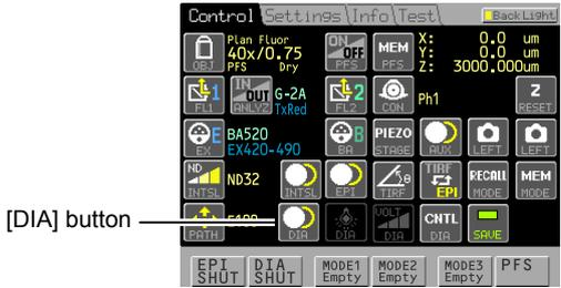
1. Pressing the [DIA] button (DIA shutter) on the [Control] screen, toggles the motorized shutter of the diascopic illumination open and closed.
