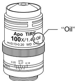
Figure 4.11-6 Oil immersion objective (example)
