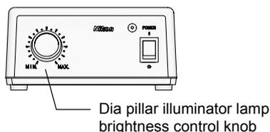
Figure 4.2-4 Dia pillar illuminator lamp brightness control knob
