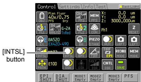
1. Pressing the [INTSL] button (Intensilight) on the [Control] screen, toggles the motorized HG fiber optic light source (Intensilight) shutter between open and closed.
