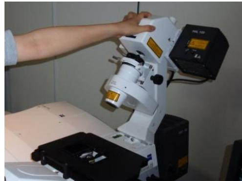
By tilting the transmitted light illuminator carrier, users can easily access the sample holder and set samples. Please hold a support, **do not** hold the halogen lamp house or the detector for transmitted light. During observation, the carrier must be moved back to the original position.
