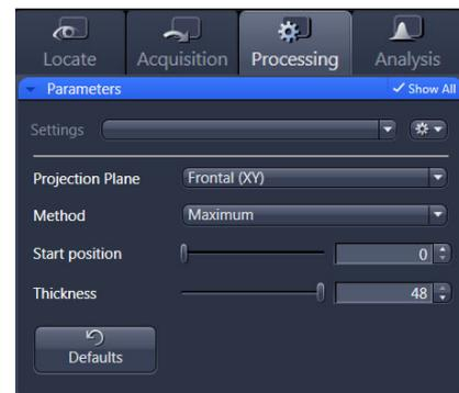
Fig.46 Orthogonal Projection
